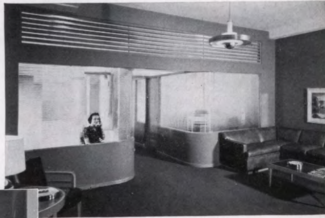
ABOVE: Screens of Louvrex with bent corners indicate how this decorative medium lends itself to modern streamlining. This is the Reception Room of the Portis Hat Company, Chicago. James F. Eppenstein, Architect, Chicago.
